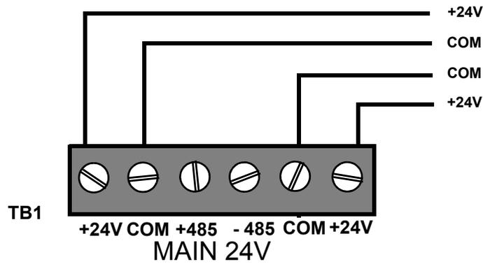
**Figure 2.11 Connecting to the Main 24 Output TB1, Example 2**
