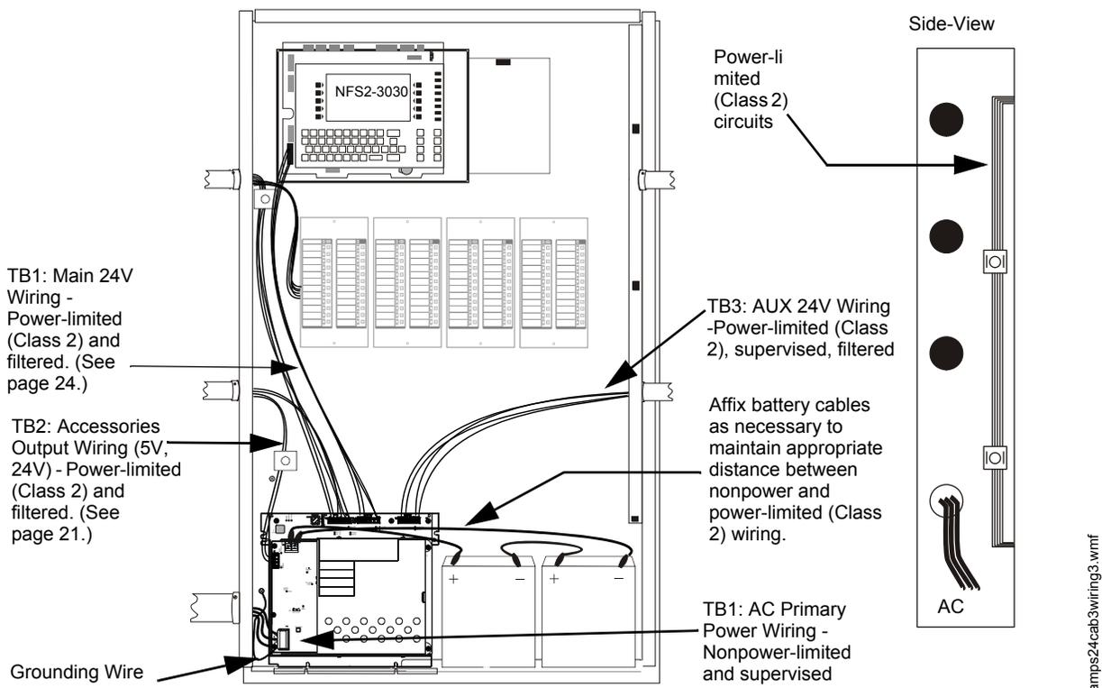
**Figure 2.7 CAB-4 Series Cabinet: Power-limited (Class 2) Wiring Example**
