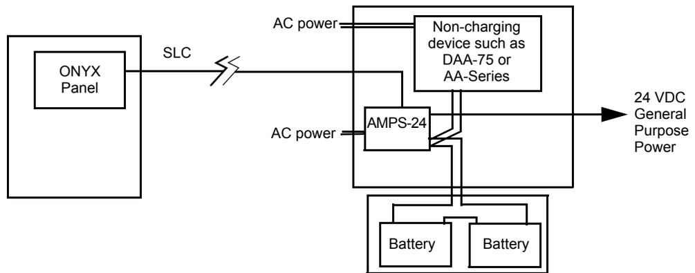
**Figure 2.12 AMPS-24 as Battery Charger/General Purpose Remote Power Supply**
