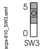
Slide the switch towards the 5, as shown in the illustration to the left, to select an initial address that ends in five. Since the rotary switch defines the decade, if the rotary switch were to point at 8, the base address in this address block would be 85.
