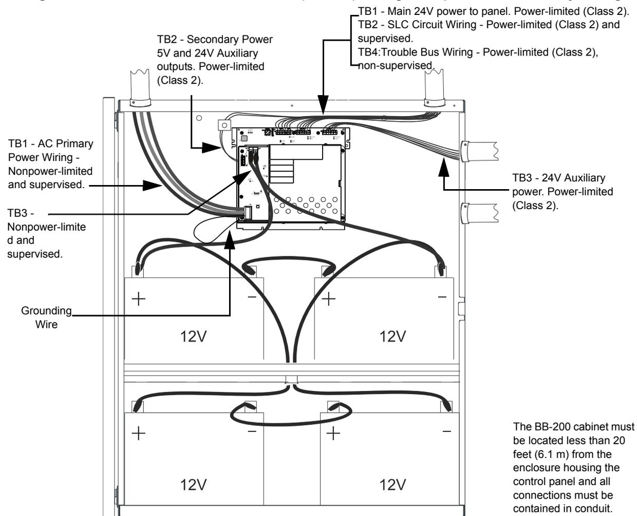
**Figure 2.9 BB-200 Cabinet: Power-limited (Class 2) Wiring Example with Four Battery Wiring**
