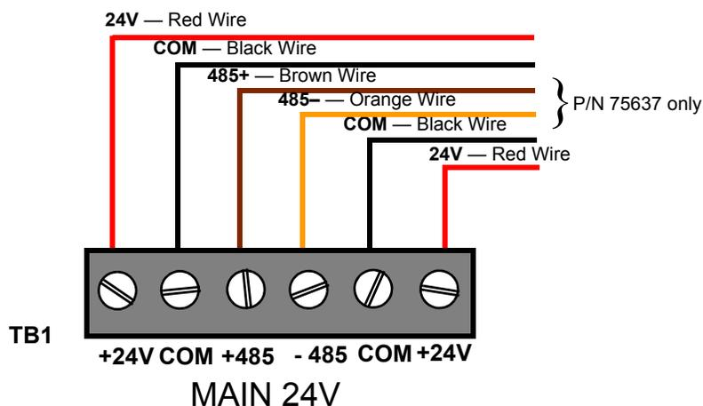
**Figure 2.10 Connecting to the Main 24 Output TB1, Example 1**
