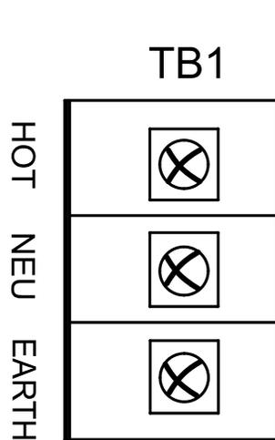
Figure 2.17 AC Power Connection
